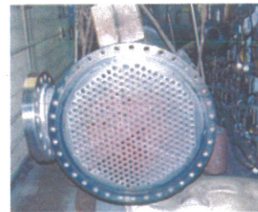
This heat exchanger exhibits multiple cracks at the flange bolt holes because design did not accommodate severe thermal transients
